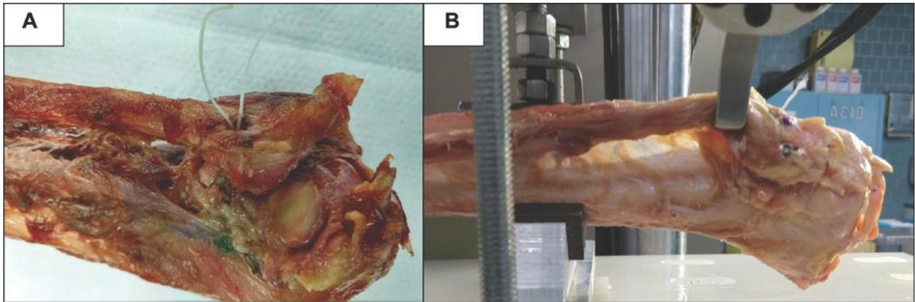
**Figure 5.** Photographs depicting failure modes after loading to failure. (A) The button was pulled into the tunnel of the fibular head, which was severely dislocated in 75% of cases. (B) Fracture or dislocation occurred in 25% of cases.
